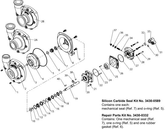
NOTE: When ordering parts, give QUANTITY, PART NUMBER, DESCRIPTION, and COMPLETE MODEL NUMBER. Reference numbers are used ONLY to identify parts in the drawing and are NOT to be used as order numbers. used as order numbers.
