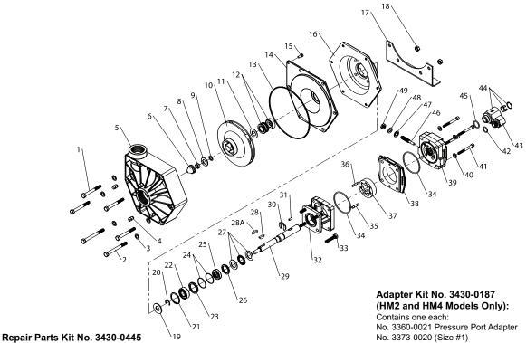
Contains: One o-ring (Ref. 13), one rubber gasket (Ref. 11), one mechanical seal (Ref. 12), one gasket (Ref. 8) and one washer (Ref. 9).
