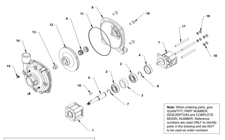
Note: Mechanical Seal Ref. 9 is not available outside of the kit form. For replacement seal, order Kit #3430-0332 or Kit #3430-0589 for Model 9302CT-GM1 and Kit #3430-0589 for
