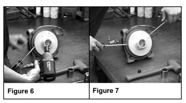
Once nut [and washer] is removed, place a screwdriver on each side behind the Impeller and pry away from the Mounting Flange (See Figure 7). Remove Woodruff Key from the Shaft. Remove O-ring from the Mounting Flange.
