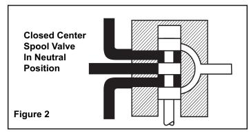
The Closed Center Valve (See Figure 2) is used with variable displacement pumps. The flow is completely shut off in the neutral position, causing the pump stroke to adjust to zero flow. The flow stops, but the pump maintains a static pressure up to the valve.
