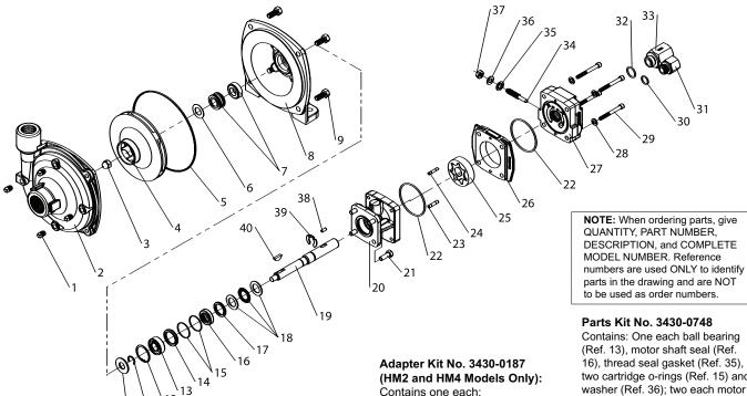
Repair Parts Kit No. 3430-0332 Contains: One o-ring (Ref. 5), one rubber gasket (Ref. 6), and one mechanical seal (Ref. 7).
