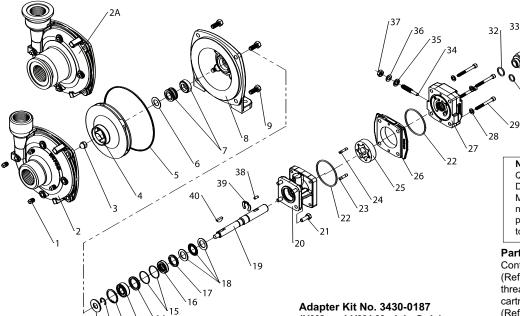
Repair Parts Kit No. 3430-0332 Contains: One o-ring (Ref. 5), one rubber gasket (Ref. 6), and one mechanical seal (Ref. 7). Silicon Seal Kit No. 3430-0589 Contains one each: 1720-0083 o-ring (Ref. 5)
