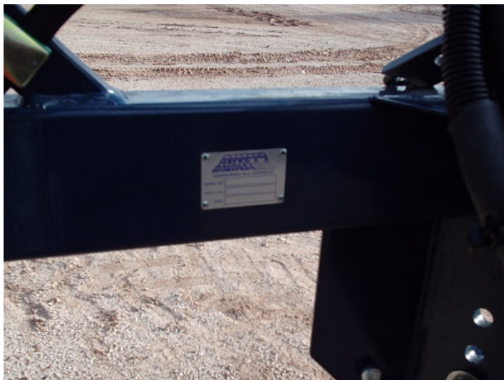
Serial Number – located on the inside of the drawbar
