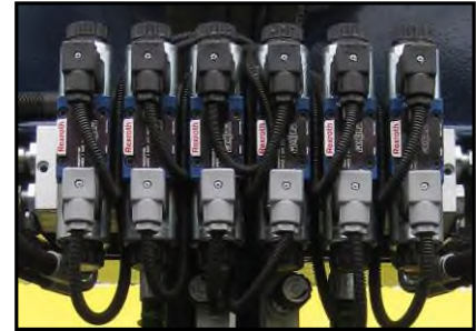
Open Centre Solenoid Spool Valve
