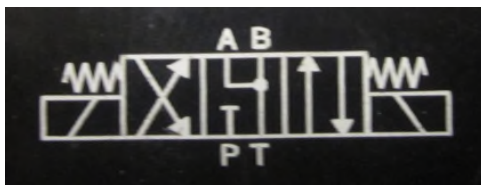
Closed Centre Solenoid Spool Valve
