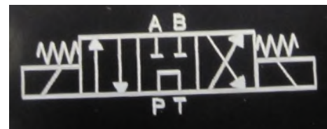
Open Centre Solenoid Spool Valve
